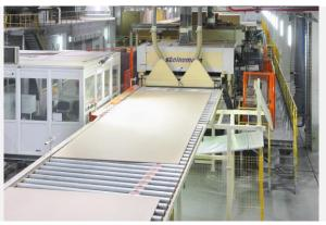
The ContiRoll press has been installed, length 35.4 meters.
