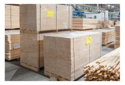
Edge-glued panels are relatively wide and thin nonstructural wood products used in the manufacture of other products such as furniture and cutting boards. They are produced from narrow pieces of wood glued along their edges to create products of greater width.
