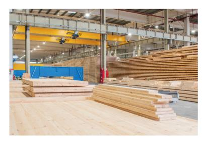
Construction line of the Rezult CLT panels (Cross-Laminated Timber) - wooden panels, manufactured from laminated layers of solid or optimized (finger-joined) sawn timber where every layer is laying in perpendicular direction to each one.
