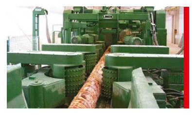
Saw line annual capacity 660000 m<sup>3</sup> of sawn timber
